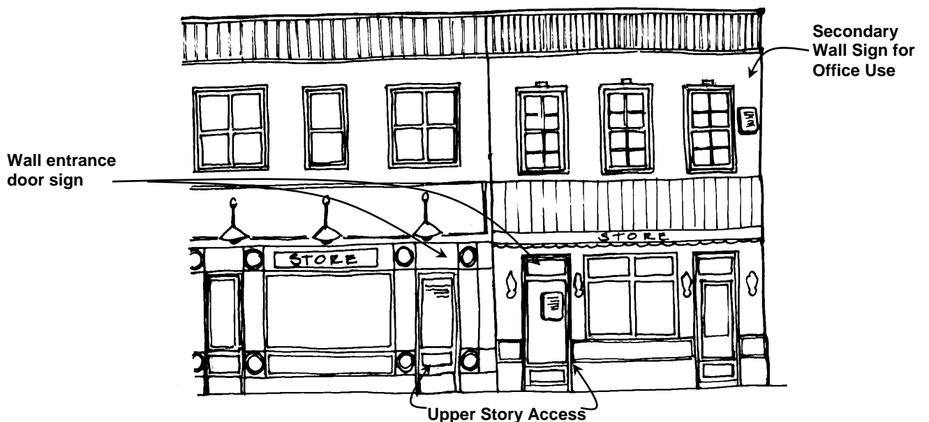
Figure 6 Wall Signs for Upper Floor Uses
