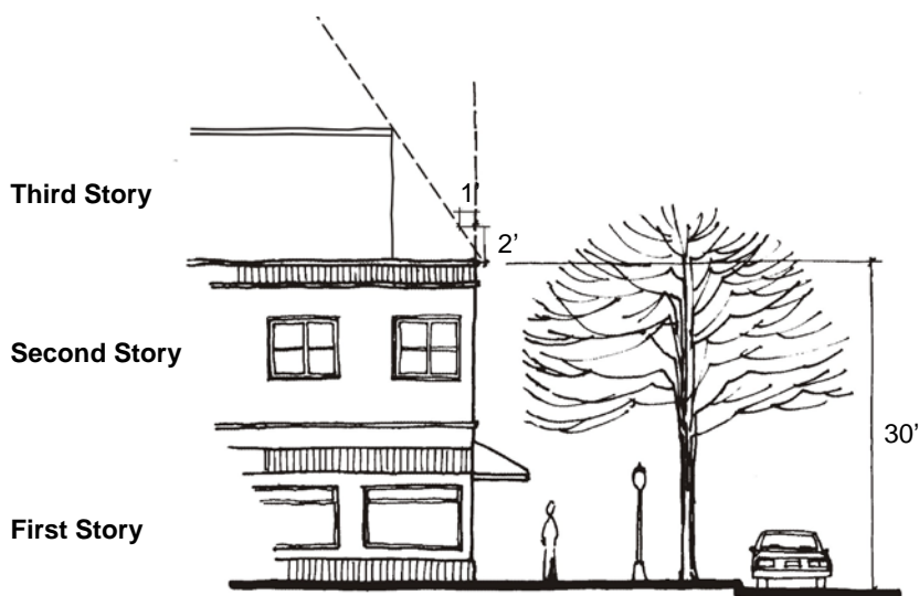
Figure 2 Stepped-Back Height Requirements
